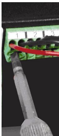
Use a small screwdriver to depress wire release for insertion / removal of wire.
