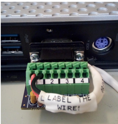
Proper installation. Label wires with their designated port.
