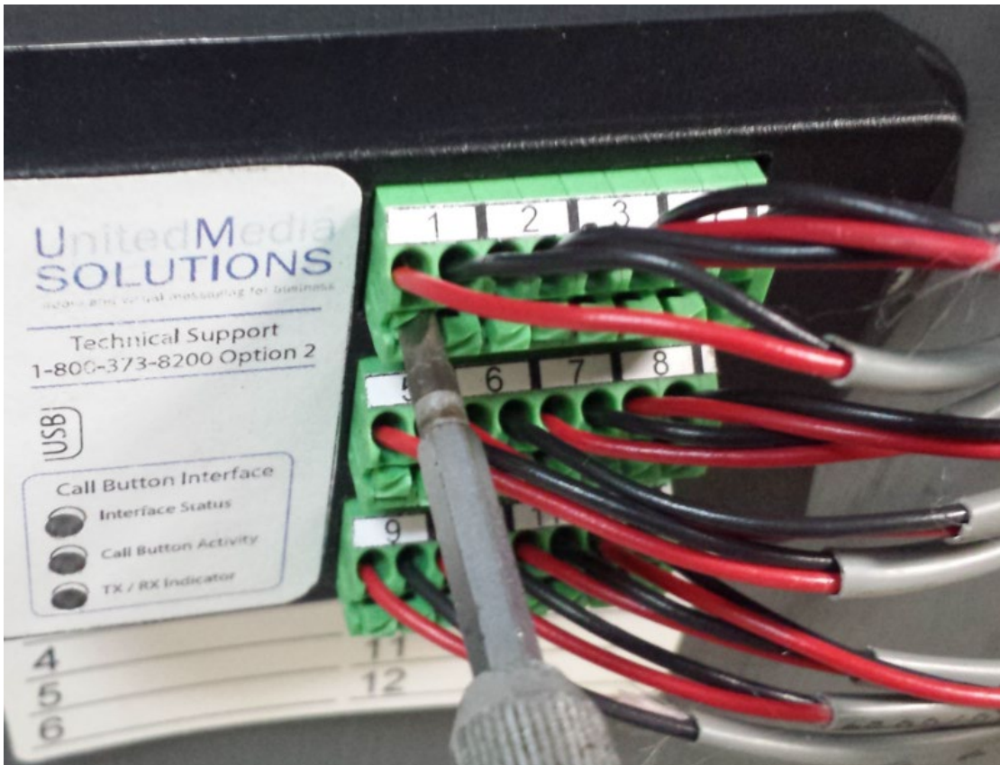
Use of small screwdriver to depress wire release for insertion / removal of wire.
