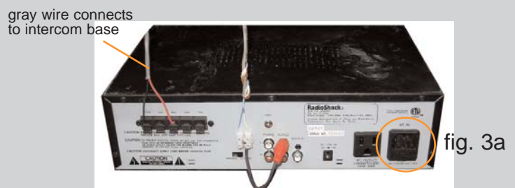
fig. 3 (back of amplifier)
